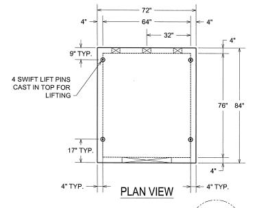
SHELTER SETS ON TOP OF GROUND, EPOXIED TO THE PURCHASER'S **CONCRETE SLAB**
