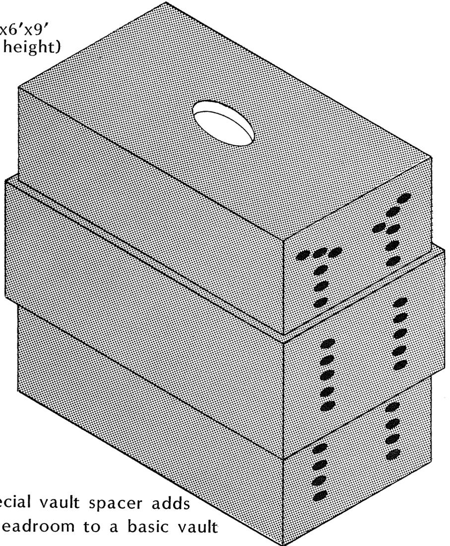
Special vault spacer adds headroom to a basic vault
