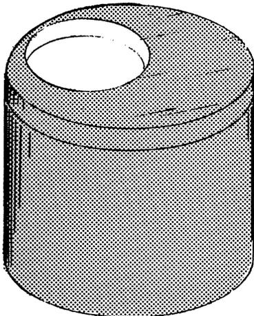
Manhole barrel section
