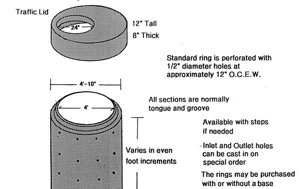
Concrete minimum strength 4000 lbs. PSI at 28 days
