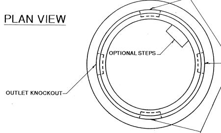
11" DIA KNOCKOUTS 1/10 HIGHER THAN OUTLET (TYPICAL OF 3)
