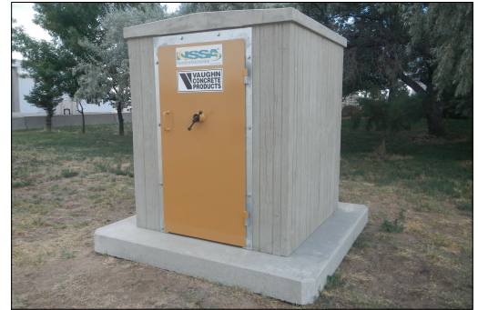
SHELTER ABOVE SHOWN WITH PRECAST CONCRETE BASE AS DETAILED ON SHEET 2 OR THE SHELTER CAN BE SOLD WITHOUT PRECAST CONCRETE BASE & PLACED ON CUSTOMER'S 9'x9'x8" THICK CAST-IN-PLACE PAD & SECURED WITH ¾" ANCHORS
